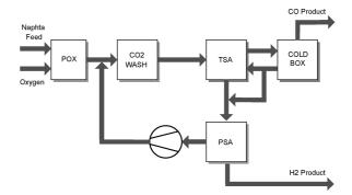
Figure 4. Combination of TSA and PSA in a H<sub>2</sub>/CO Plant.
