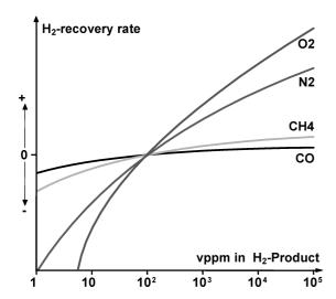
Figure 6. Hydrogen recovery vs. hydrogen purity.
