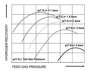
Figure 5. Influence of tail gas pressure on the hydrogen recovery rate in dependence on the feed gas pressure.
