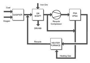
Figure 3. CO<sub>2</sub> removal from direct reduction gas.
