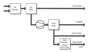
Figure 2. Combination of H<sub>2</sub>- and CO<sub>2</sub>-PSA.
